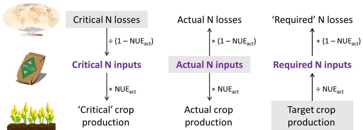
**Figure 2:** *The drivers behind the calculation of (i) actual N inputs, based on actual fertiliser consumption and livestock numbers, (ii) required N inputs, based on target crop yields and (iii) critical N inputs, based on critical N losses to air and water based on critical values for defined N indicators.*
