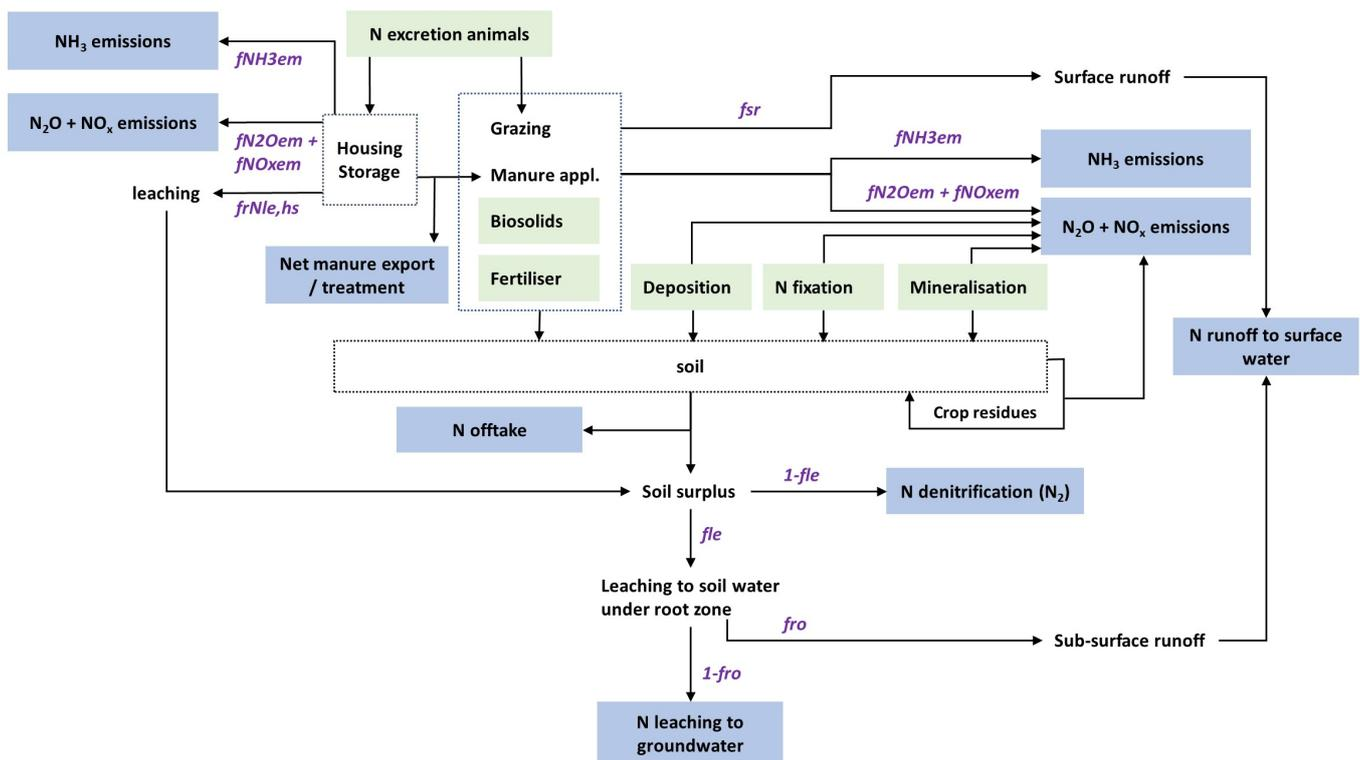
**Figure 3:** Schematic presentation of the calculated N flows in INTEGRATOR (adapted after the MITERRA-EUROPE model by Velthof *et al.*, 2009; see text for description of calculation methods). At the NCU level, the sum of total gross N inputs (green boxes) equals the sum of all N outputs (blue boxes). The sum of all green boxes equals the sum of all blue boxes.
