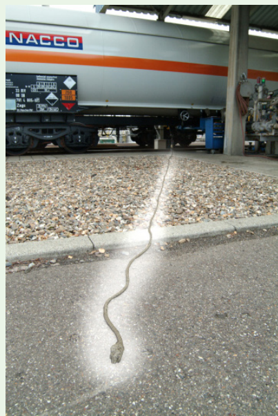
Figure 18 Connection ring and cable between the rail hook and the bottom valve of the RTC for closure of the bottom valve upon movement of the RTC
