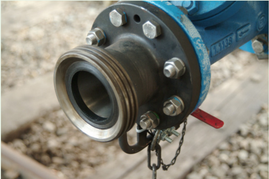
Figure 10 ACME type WECO 6000 psi Screw coupling
