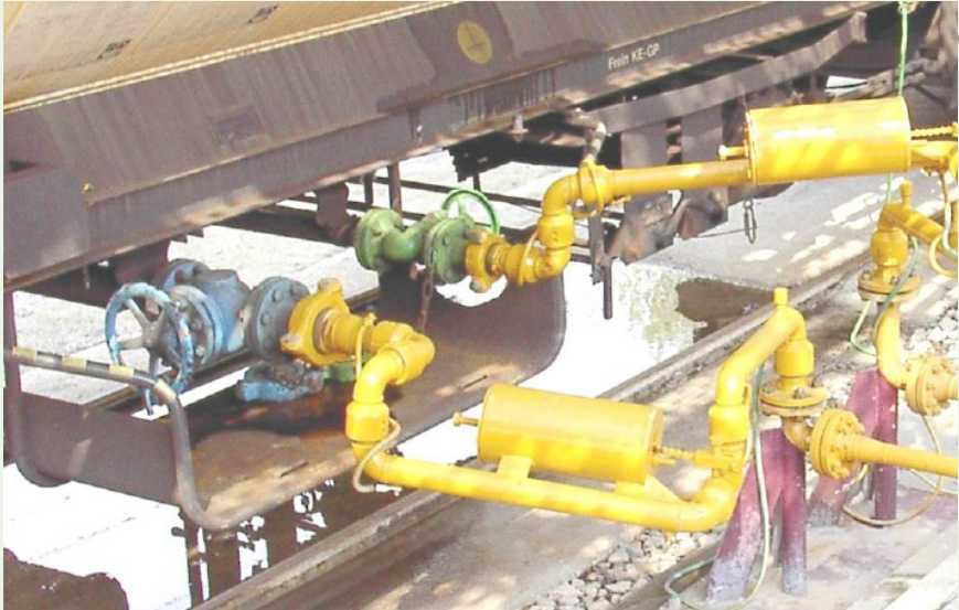
Figure 9 Screw couplings of the WECO type
