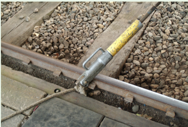
Figure 18 Connection ring and cable between the rail hook and the bottom valve of the RTC for closure of the bottom valve upon movement of the RTC
