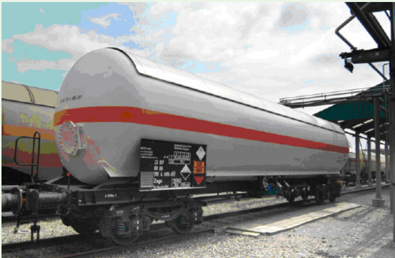
Figure 2 Typical example of an ammonia RTC showing the orange band, heat shield and identification plate
